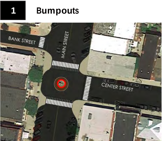
1: Bumpouts enable shorter pedestrian crossings and protect 'bear' with curb
